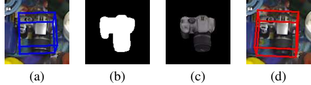
Figure 4. Refining the pose. Given a first pose estimate, shown by the blue bounding box (a), we generate a binary mask (b) or a color rendering (c) of the object. Given the input image and this mask or rendering, we can predict an update that improves the object pose, shown by the red bounding box (d).
