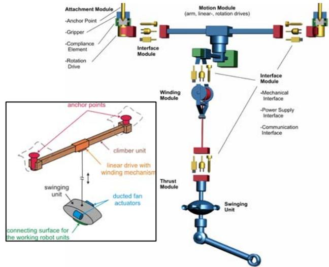
**Figure 2. Embodiment design evolution of the ACROBOTER system.**
