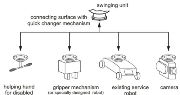
**Figure 3. ACROBOTER is a mobile service robot platform.**
