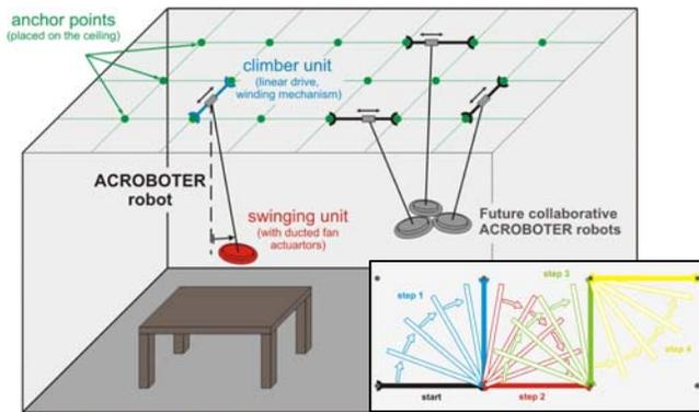
**Figure 1. Concept of the ACROBOTER platform (framed part shows the movement of the climber unit between the anchor points). The concept opens ways of collaboration of more platforms in a physically coupled configuration.**
