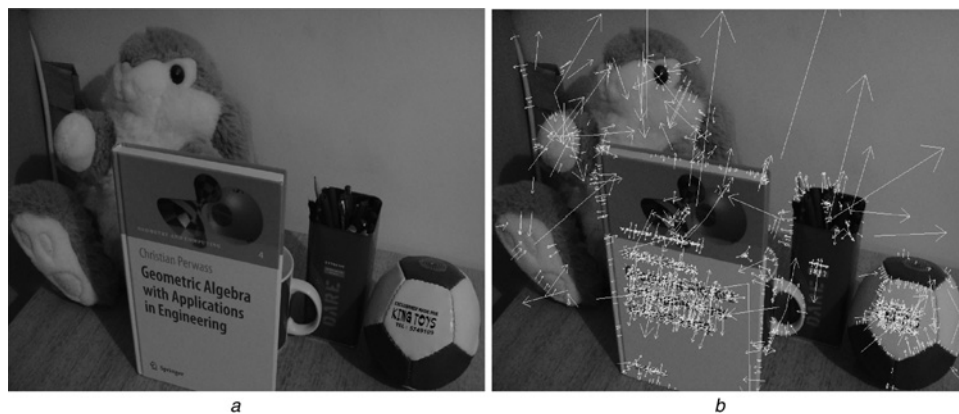
Fig. 6 System in cases of total objects' occlusions (e.g. cup) fails to estimate their depth
